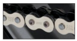
12a. After pressing the sideplate on, disassemble the chain tool and remove it from the chain. The next step is to flare out the pins heads for ZJ (Rivet type) or installing the slide clip for the FJ (Clip type) master link.
