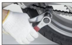
15a. Hold the hexagon part of the tool body by with a 27mm closed in wrench, and the bolt head with a 19mm closed end wrench; turn clockwise until the flare part of the pin head makes contact with the surface of the side plate.
